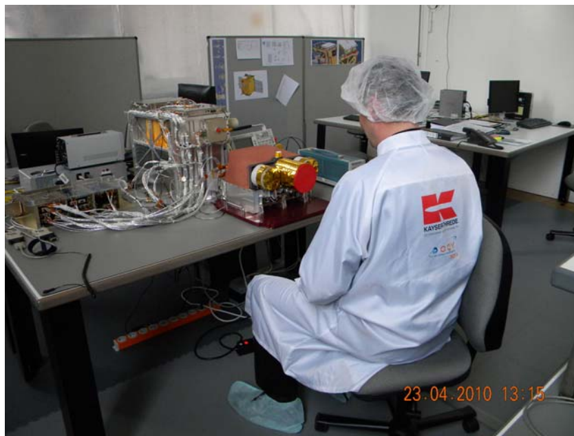
Fig. 6. Payload N15 (Infrared Camera) during acceptance testing
