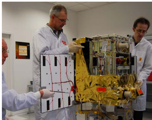
Fig. 16. Final satellite integration (Picture shows STM)
