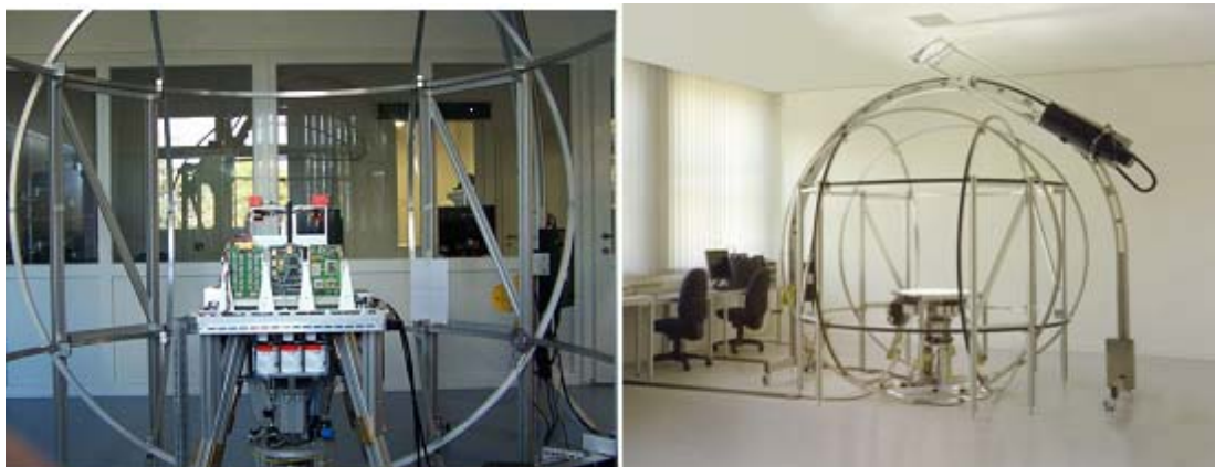
Fig. 15. EM AOCS (left) on AOCS test bed (right)
