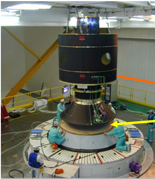
Fig. 2: MAQSAT-B2 as lower passenger on L521, a 3,5t fully representative test satellite carrying experiments on board and the mini satellite SloshSat on top.
