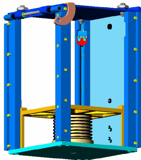
Figure 13: Single PicoSat Launch Device SPL (by courtesy of Astro Feinwerktechnik)
