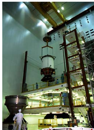
Figure 3: Ariane 502 (left) with dummy payloads MAQSATB (middle) and MAQSATH during integration onto the launcher
