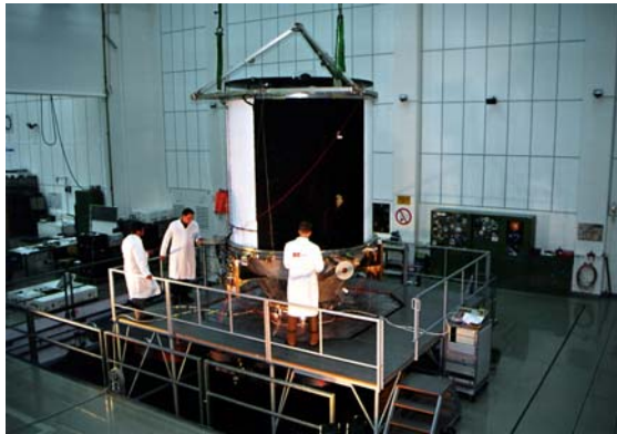
Figure 1: Structural verification of MAQSATH
