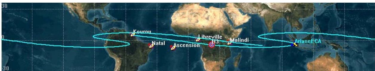
FIG 5: Ground Track of L521 out of MAQSAT-B2 mission analysis
