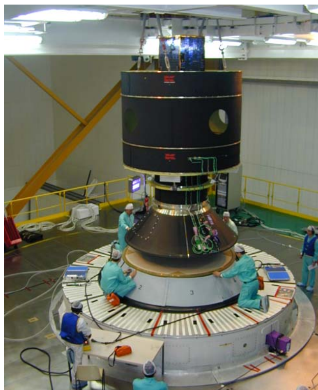
FIG 24. Integration of MAQSAT-B2 to the launcher
