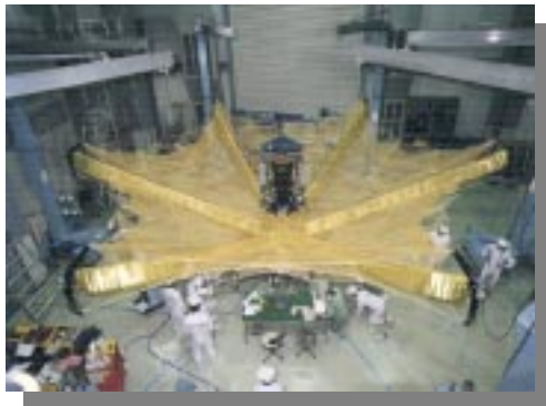
Tension truss antenna reflector, Japan
